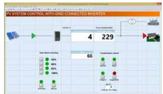
SCADA with derating of photovoltaic inverter
