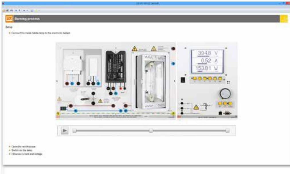
Experiment: How fluorescent lights work and how to connect them via conventional ballast.
